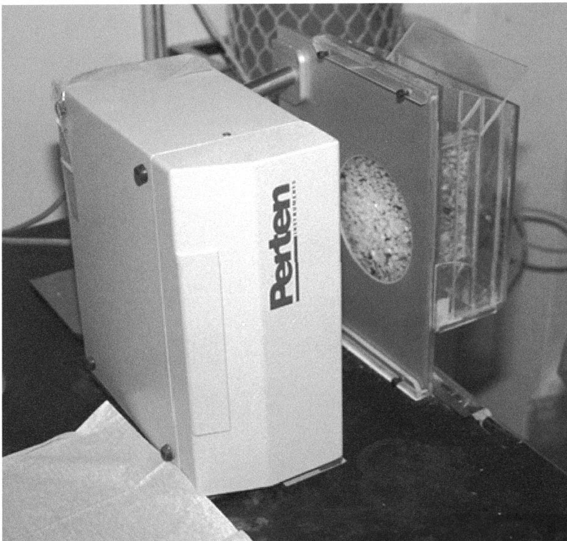
Figure 1. InGaAs/silicon dual-diode-array NIR spectrometer and hopper accessory for rapid loading and measurement of the reflectance of a large surface area of each cereal food product.
